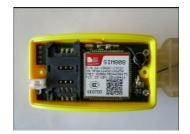
Unscrew the two screws carefully, with the screwdriver provided in the package. Make sure to always use the screwdriver provided. Open the plastic cover carefully, by paying attention to the battery wires and insert the SIM card as shown on the photo above. Then, close tight the plastic cover and screw the two screws. Make sure you close the plastic cover tight so the tracker is waterproof.
